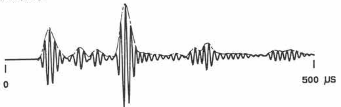
Fig. 6: Echo of a single, simulated dolphin echolocation click after its reflection from a water filled steel sphere. After AU (1993).
