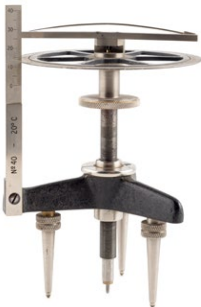
Spherometer MHS 2647 Steel, SIP, Geneva, 20th century
