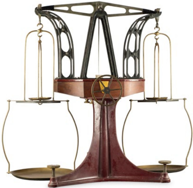
Laboratory precision scales MHS 718 Steel, cast iron, brass, Deleuil, Paris, 19th century
