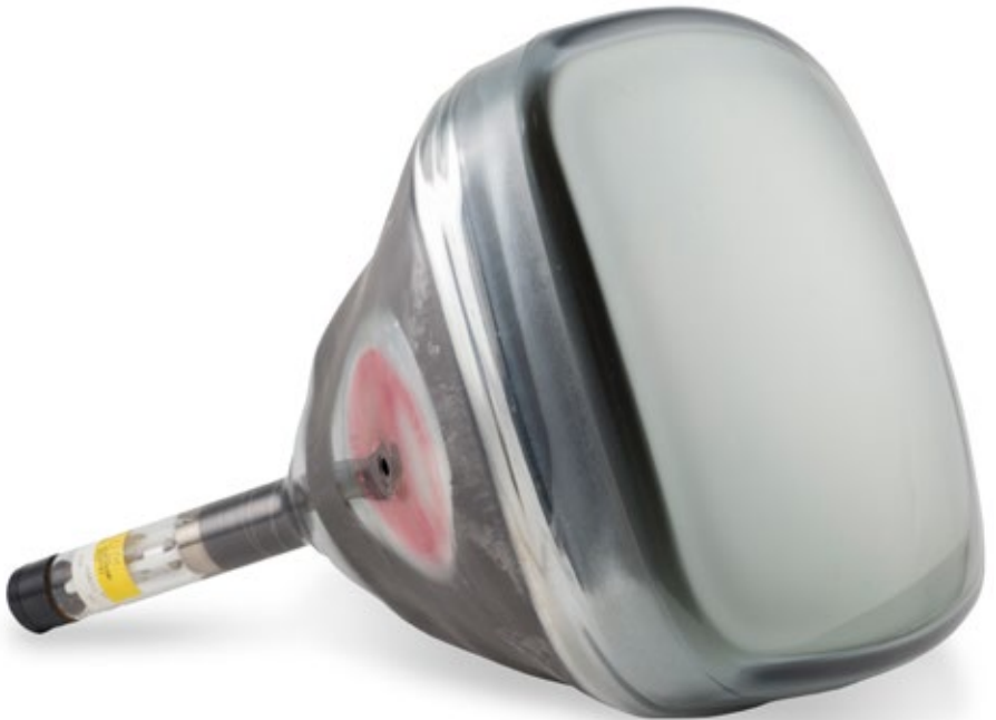
Television cathode ray tube MHS 2725 Steel, aluminium, glass
