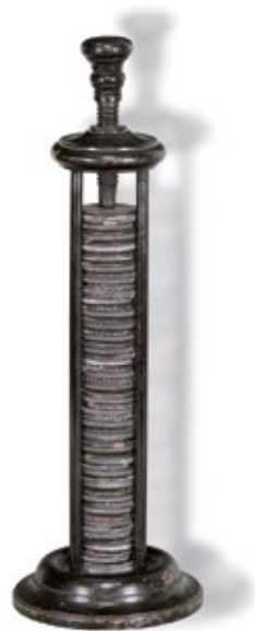
Voltaic Pile MHS 373 Wood, cooper, zinc, glass, Volta, vers 1802
