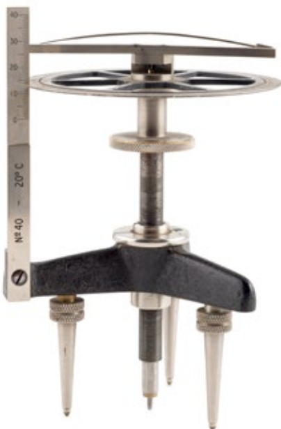
Spherometer MHS 2647 Steel, SIP, Geneva, 20th century
