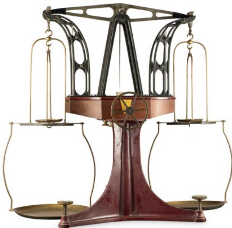
Laboratory precision scales MHS 718 Steel, cast iron, brass, Deleuil, Paris, 19th century
